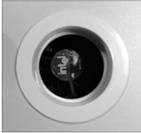
Figure 21.26. Peering through the duct to measure the clearance between the duct and processor heatsink.
