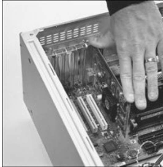
Figure 20.26. This photo shows a video adapter being inserted into the slot. Motherboard courtesy of Intel Corporation.
