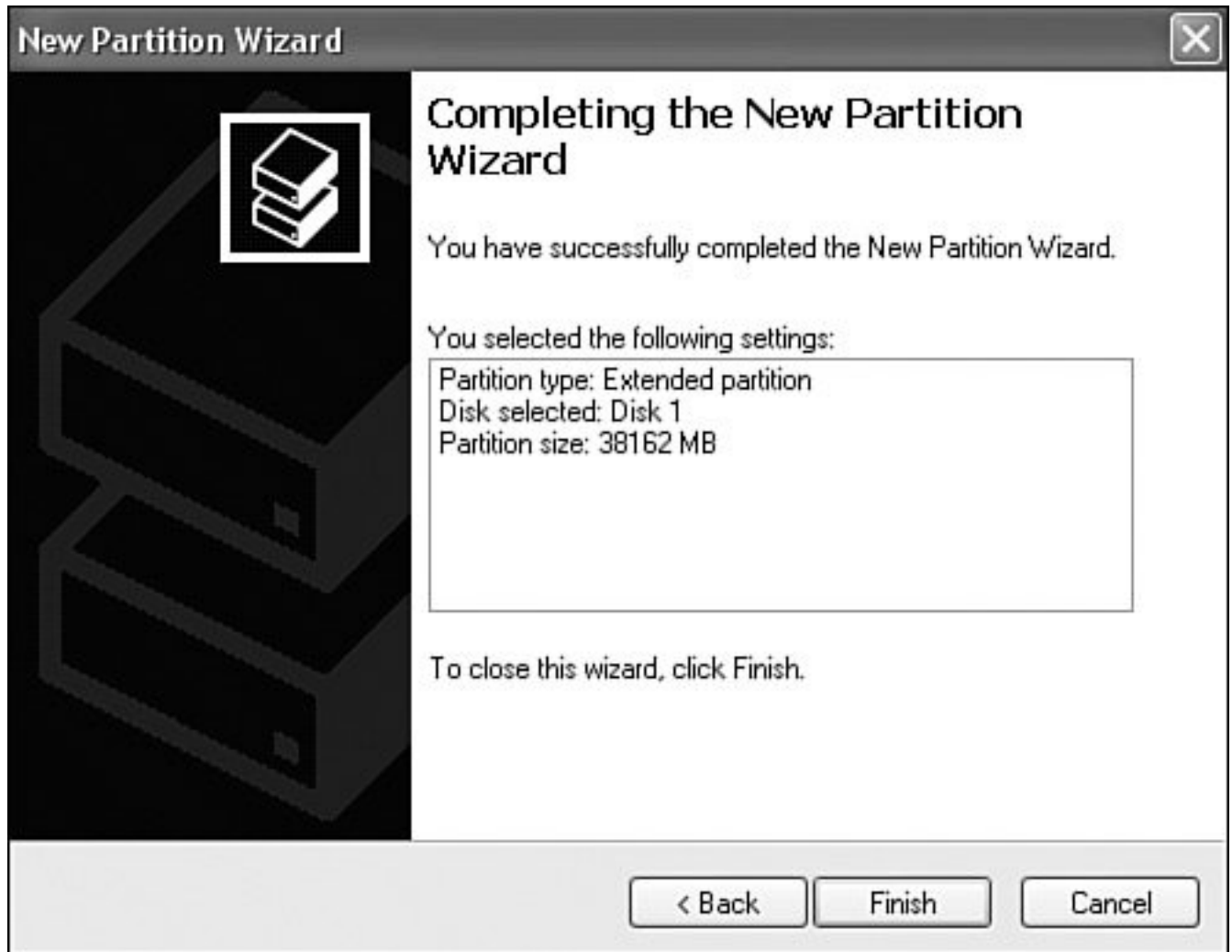
Figure 12.9. The New Partition Wizard prepares to create an extended partition from Disk 1.
