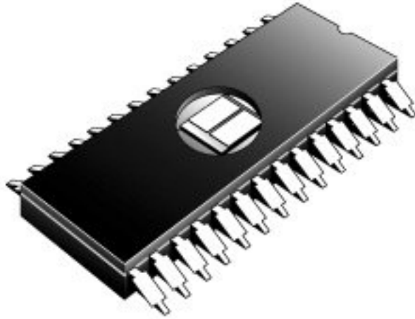
Figure 5.4. An EPROM showing the quartz window for ultraviolet erasing.
