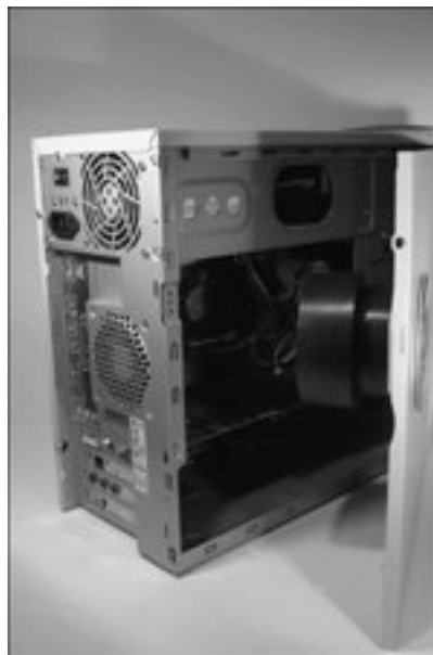
Figure 21.27. Side cover with the duct being reinstalled on the chassis.
