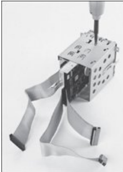
Figure 12.3. A typical hard disk mounted in a removable drive cage.
