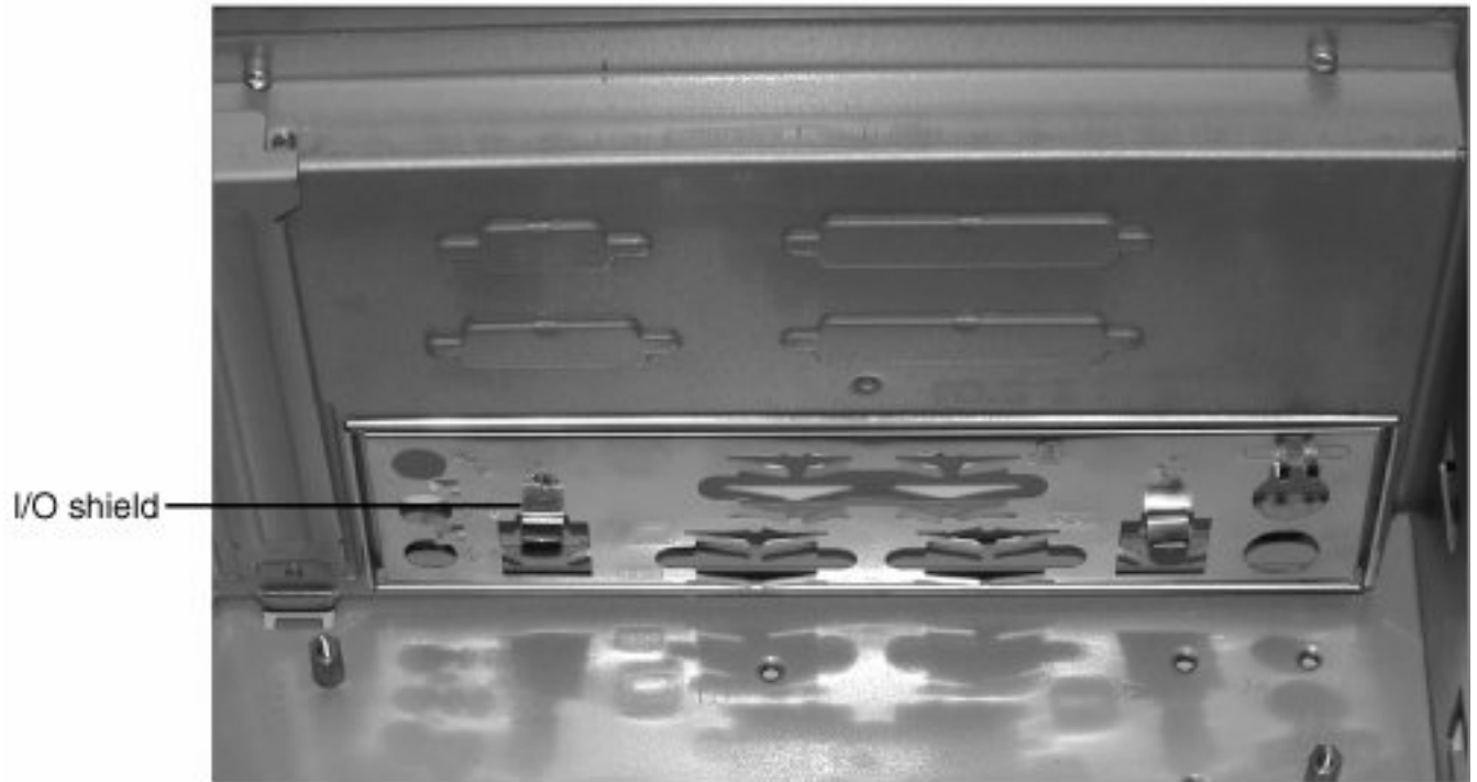
Figure 20.15. The I/O shield after being snapped into place in the chassis.
