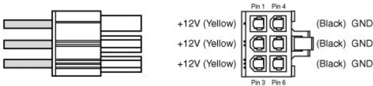
Figure 19.36. PCI Express x16 Graphics 150W power connector.
