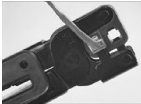
Figure 18.15. Firmly squeeze the crimping tool to attach the connector to the cable.
