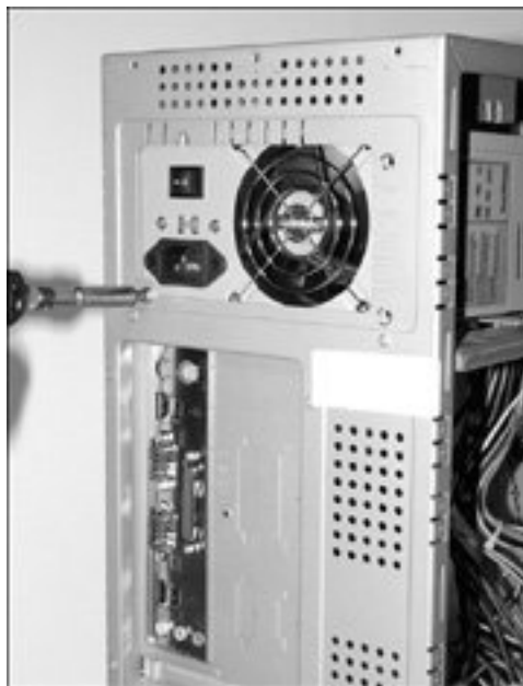
Figure 20.19. Installing the screws to retain the power supply.
