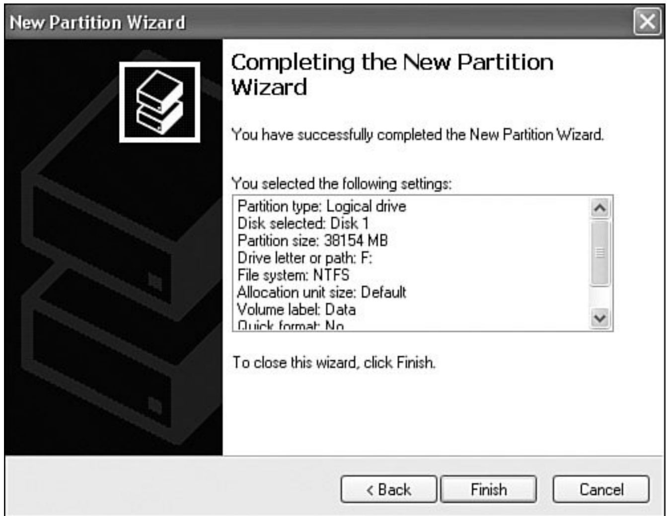
Figure 12.10. The New Partition Wizard prepares to format a logical drive on Disk 1 with the options shown.
