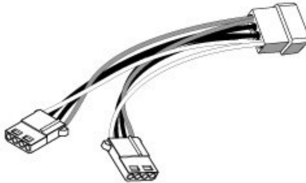
Figure 19.32. A common Y-adapter power cable.
