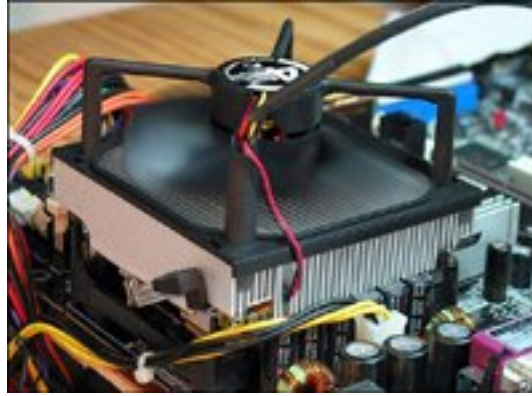
Figure 21.12. The Arctic Cooling Super Silent 4 Ultra TC CPU fits socket 478 CPUs. (Photo courtesy of Mike Chin/SilentPCReview.com.)
