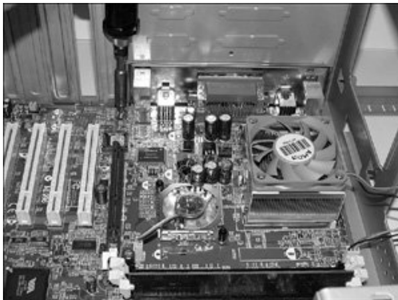
Figure 20.17. Installing the screws that hold the motherboard to the chassis.
