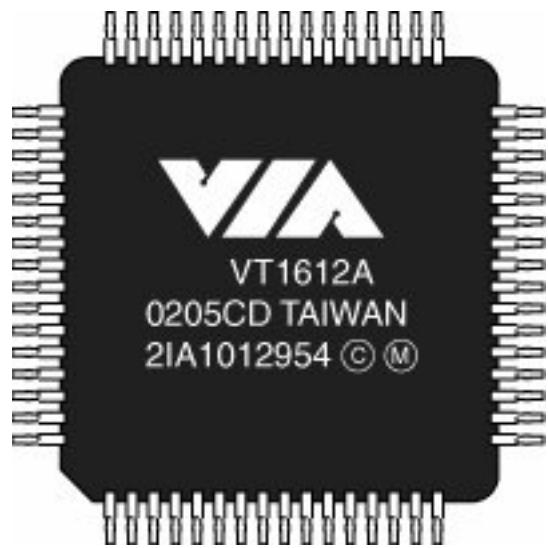
Figure 14.8. The VIA VT1612A is a typical AC'97 2.2compliant codec chip. Photo courtesy of VIA Technologies, Inc.
