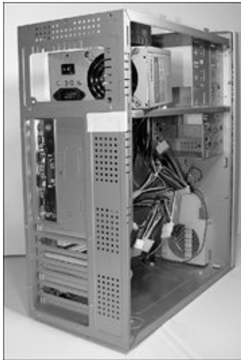
Figure 20.18. Installing the power supply into the chassis.
