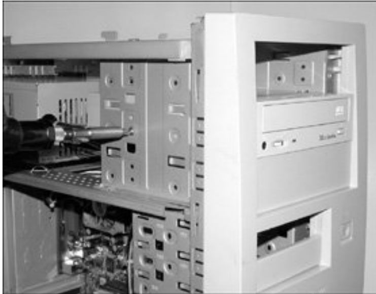
Figure 20.23. Secure the drive to the chassis using four screws.
