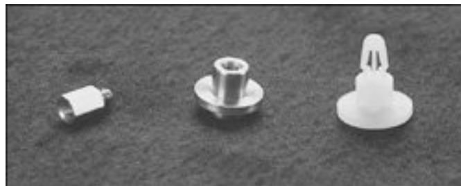
Figure 20.11. Various types of motherboard standoffs, used to support the board when installed in the chassis or motherboard tray.
