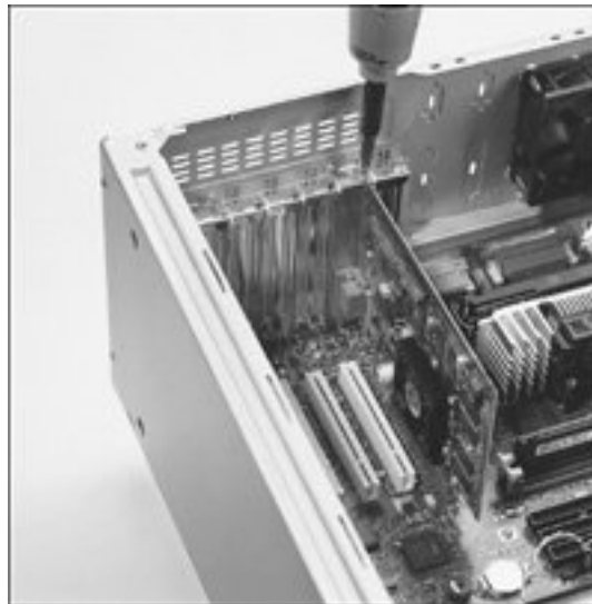
Figure 20.27. Installing the screw to retain the card. Motherboard courtesy of Intel Corporation.
