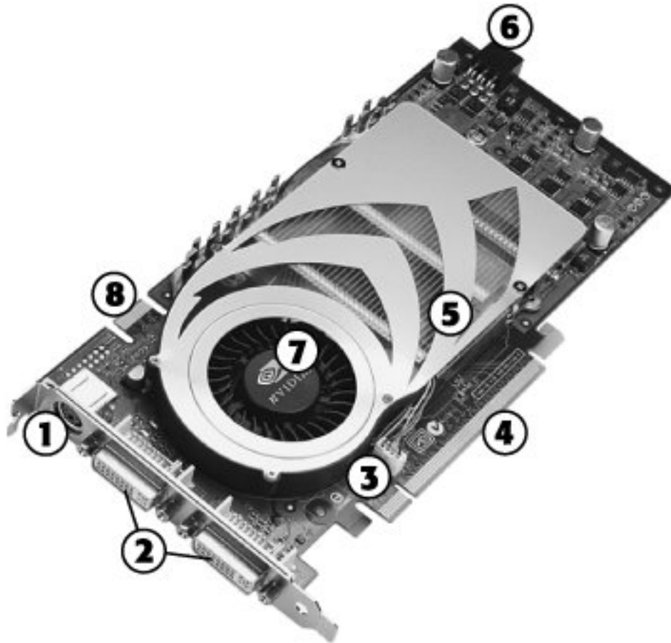
Figure 13.14. A typical example of a high-end video card based on the NVIDIA GeForce 7800 GTX, a GPU optimized for gaming and dual-display support.
