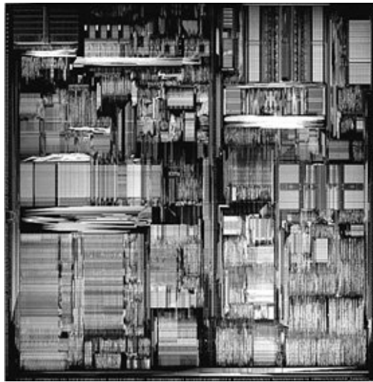
Figure 3.42. Pentium Pro processor with 256KB L2 cache (the cache is on the left side of the processor die). Photograph used by permission of Intel Corporation.
